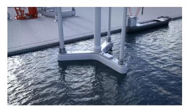
Once launched, the substructure and turbine will be elevated and checked out dockside. Many pre-commissioning activities can be conducted with convenient near-shore access. Once completed, the system can be towed to a nearby holding area to await favorable installation conditions or it can be towed directly to the wind farm and installed.
